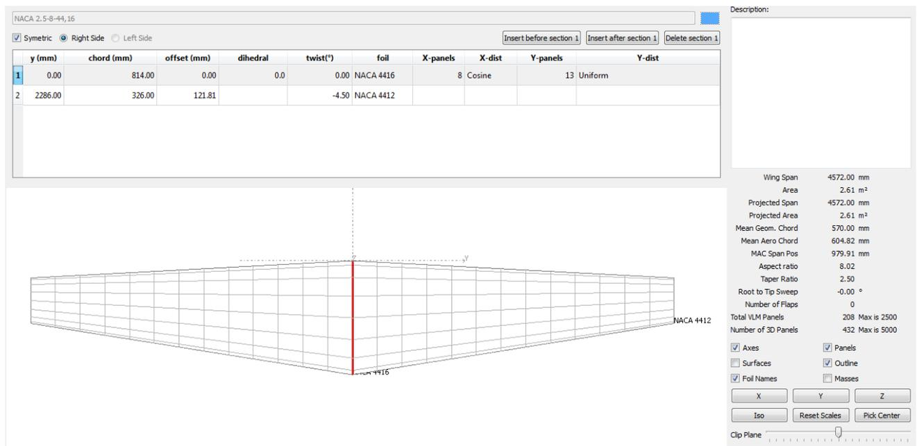
Wing NACA 3.5-12-44,22.1 has been analyzed for Re=4e6 and M=0.19.
